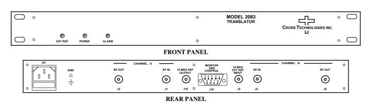
FIGURE 1.1 Model 2083-0372 Front & Rear Panels
