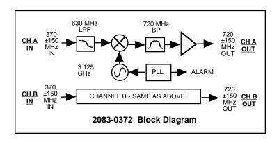
FIGURE 1.2 Model 2083-0372 Block Diagram
