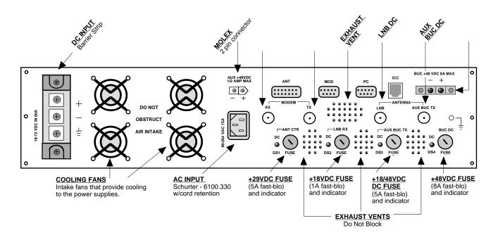
FIGURE 2.2 Rear Panel Outputs
