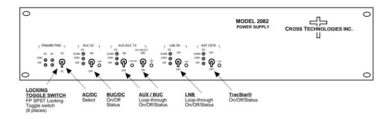
FIGURE 2.3 Front Panel Controls and Indicators
