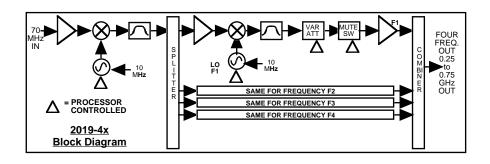
FIGURE 1.2 Model 2019-4x Upconverter, Block Diagram
