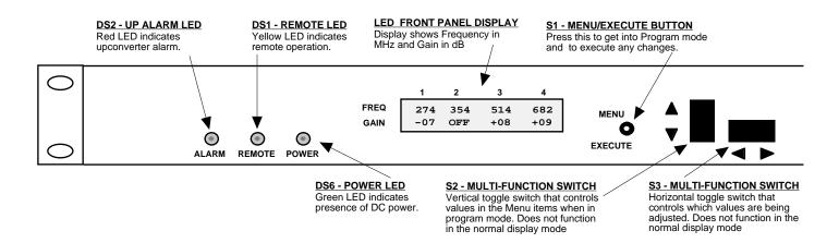
FIGURE 2.2 2019-4x Front Panel Controls and Indicators
