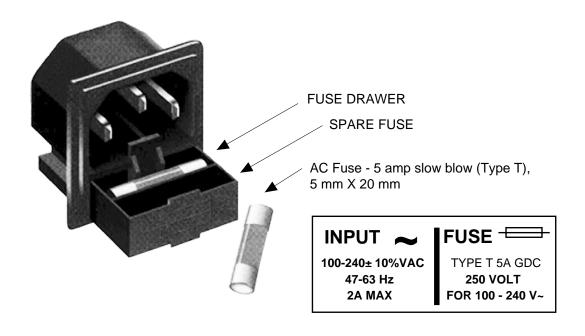
Figure 2.3 Fuse Location and Spare Fuse
