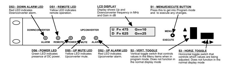
Figure 2.2 Model 2017-95 Front Panel Controls and Indicators
