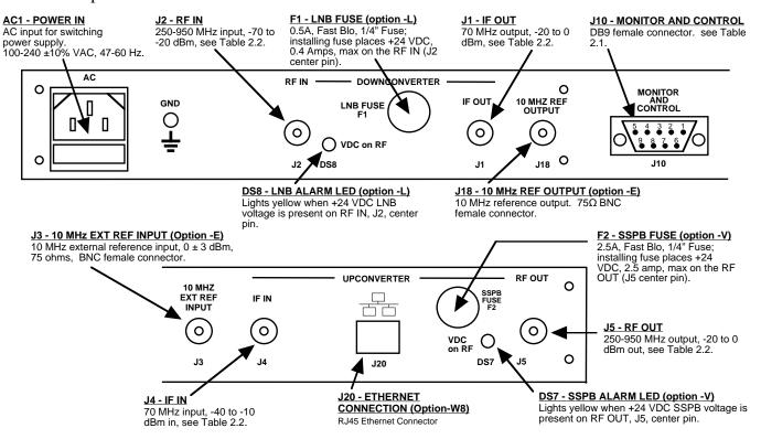
Figure 2.1 Model 2017-95 Rear Panel I/O's
