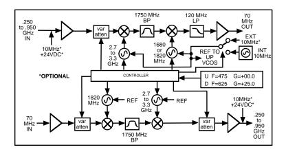
Figure 1.2 Model 2017-95 Up/Downconverter Block Diagram
