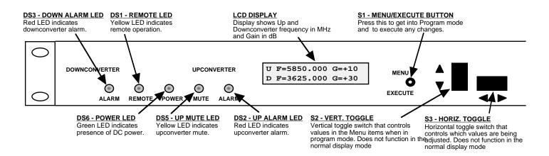
**Figure 2.2 Front Panel Controls and Indicators**
