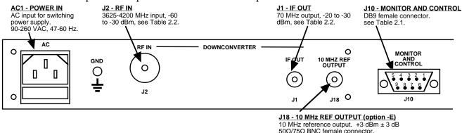
10 MHz reference output. +3 dBm  $\pm$  3 dB  $50\Omega/75\Omega$  BNC female connector.
