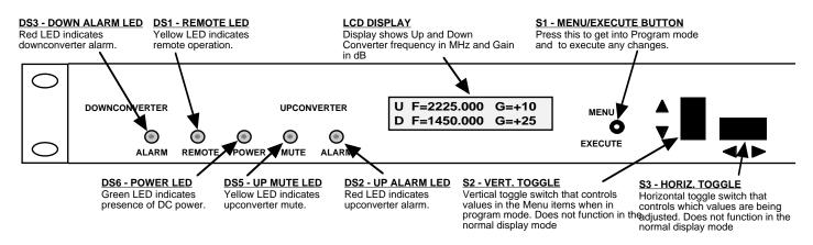
Figure 2.2 Model 2017-35 Front Panel Controls and Indicators
