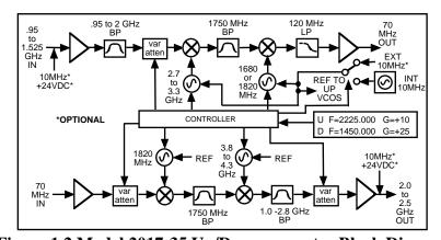
Figure 1.2 Model 2017-35 Up/Downconverter Block Diagram
