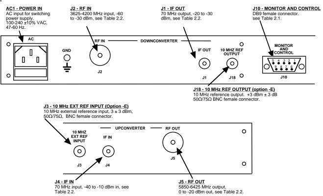
Figure 2.1 Model 2017-35 Rear Panel I/O's
