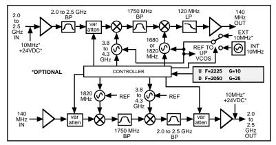
Figure 1.2 Model 2017-26 Up/Downconverter Block Diagram
