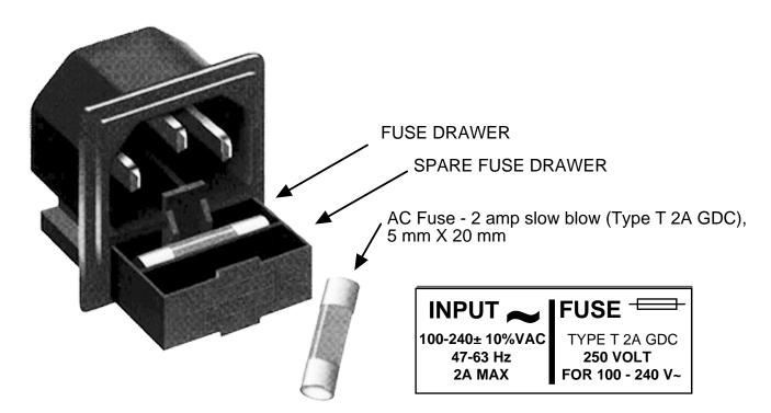
Figure 2.3 Fuse Location and Spare Fuse
