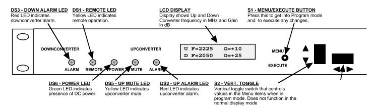
Figure 2.2 Model 2017-26 Front Panel Controls and Indicators
