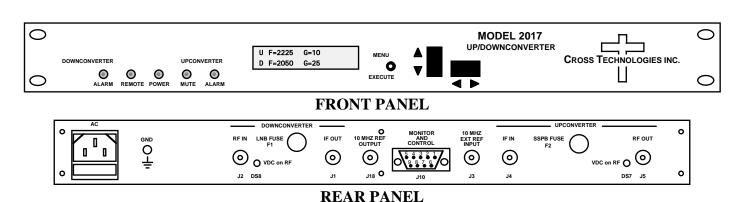
Figure 1.1 Model 2017-26 Front and Rear Panels
