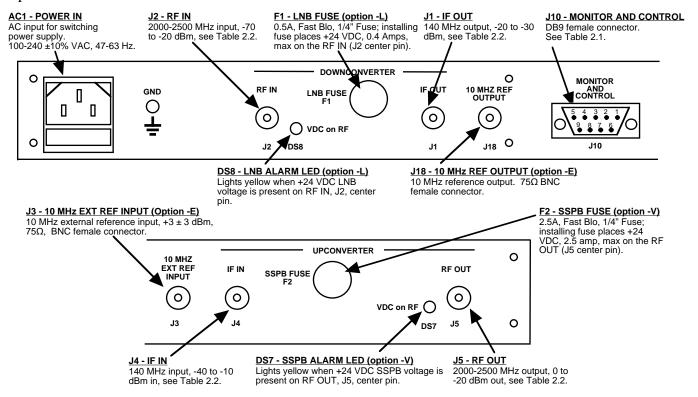
Figure 2.1 Model 2017-26 Rear Panel I/O's
