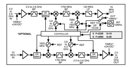
Figure 1.2 Model 2017-25-02 Up/Downconverter Block Diagram
