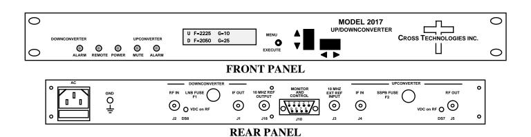
Figure 1.1 Model 2017-25-02 Front and Rear Panels
