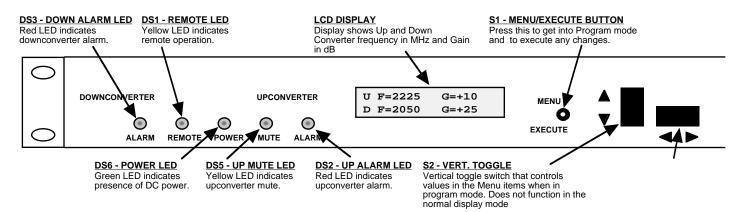
Figure 2.2 Model 2017-25-02 Front Panel Controls and Indicators
