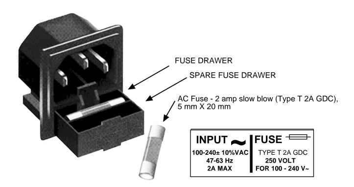
**Figure 2.3 Fuse Location and Spare Fuse**
