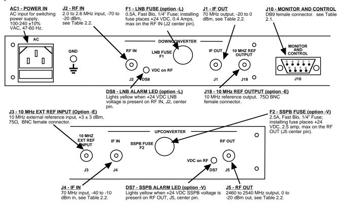
Figure 2.1 Model 2017-25-02 Rear Panel I/O's
