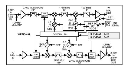
Figure 1.2 Model 2017-25-01 Up/Downconverter Block Diagram
