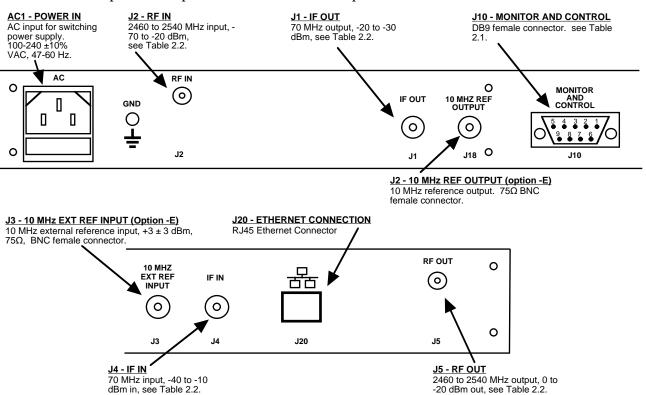
Figure 2.1 Model 2017-25-01 Rear Panel I/O's
