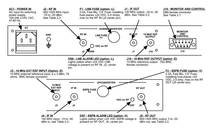
Figure 2.1 Model 2017-05 Rear Panel I/O's
