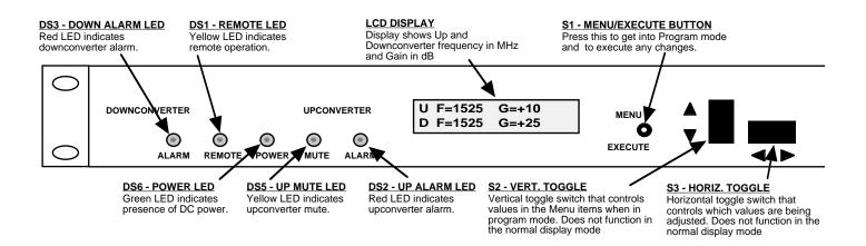
Figure 2.2 Model 2017-05 Front Panel Controls and Indicators
