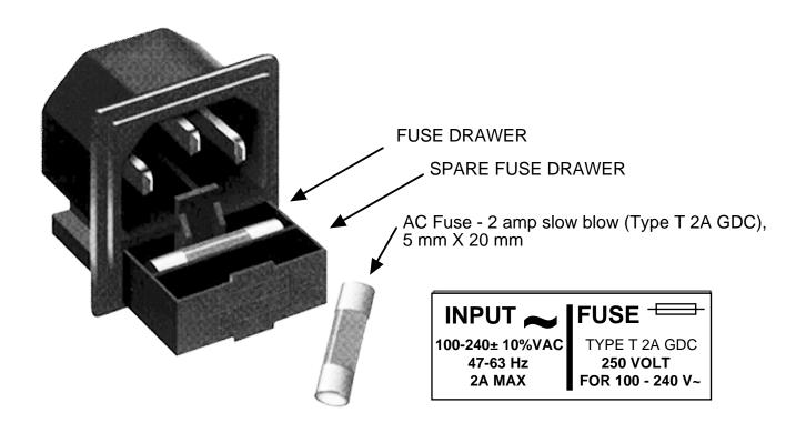
**Figure 2.3 Fuse Location and Spare Fuse**
