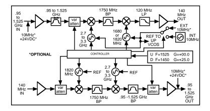
Figure 1.2 Model 2017-05 Up/Downconverter Block Diagram
