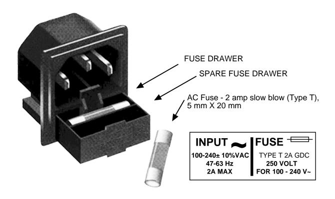
**Figure 2.3 Fuse Location and Spare Fuse**
