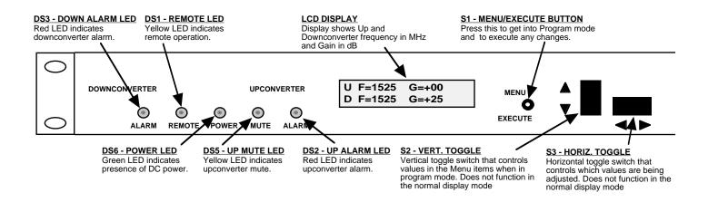
Figure 2.2 Model 2017-05A Front Panel Controls and Indicators
