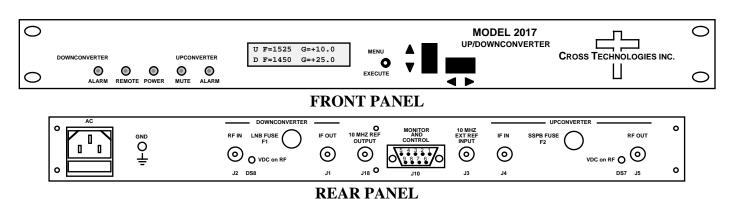
Figure 1.1 Model 2017-05A Front and Rear Panels
