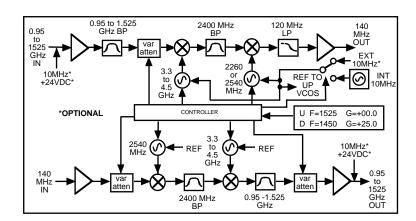
Figure 1.2 Model 2017-05A Up/Downconverter Block Diagrams
