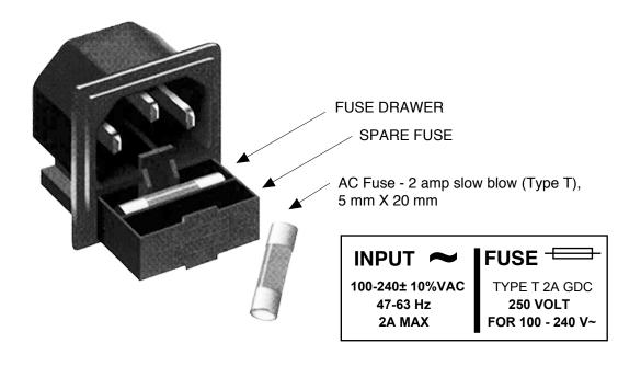
Figure 2.3 AC Fuse Location and Spare Fuse
