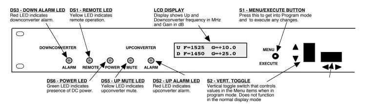
Figure 2.2 Model 2017-04 Front Panel Controls and Indicators
