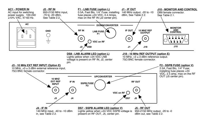
Figure 2.1 Model 2017-04 Rear Panel I/O's
