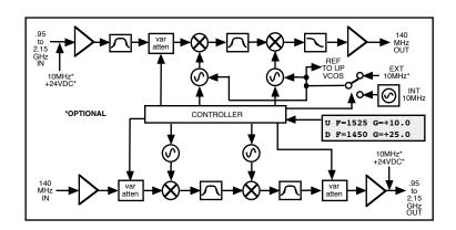
Figure 1.2 Model 2017-04 Up/Downconverter Block Diagram
