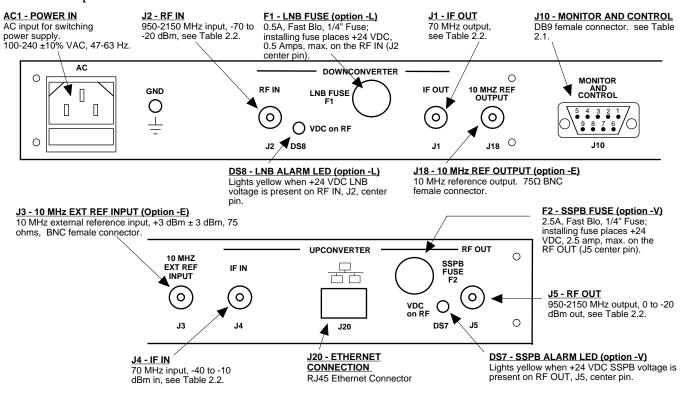
Figure 2.1 Model 2017-02 Rear Panel I/O's
