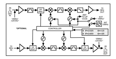
Figure 1.2 Model 2017-02 Up/Downconverter Block Diagram
