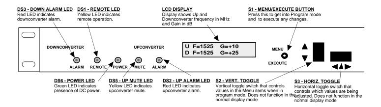
Figure 2.2 Model 2017-02 Front Panel Controls and Indicators
