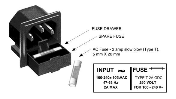
Figure 2.3 Fuse Location and Spare Fuse
