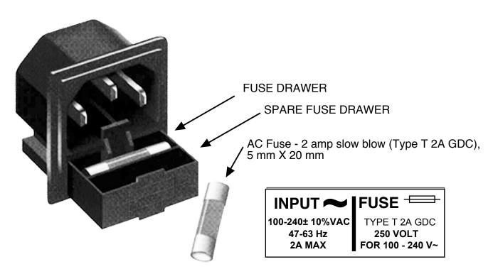
FIGURE 2.3 Fuse Location and Spare Fuse
