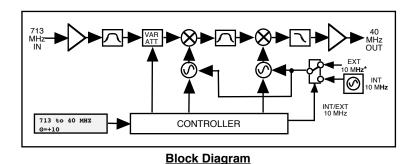
FIGURE 1.2 Model 2016-75-40 Downconverter Block Diagram
