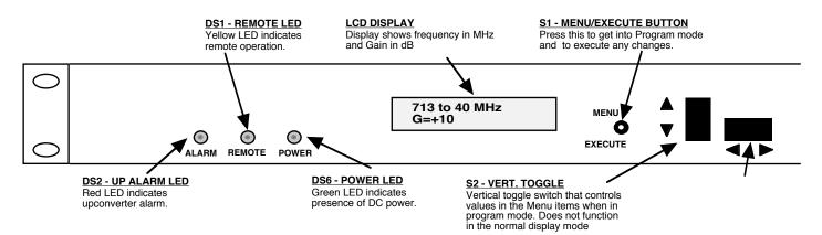
FIGURE 2.2 2016-75-40 Front Panel Controls and Indicators
