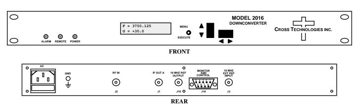
FIGURE 1.1 Model 2016-37 Front and Rear Panels
