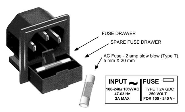
FIGURE 2.4 Fuse Location and Spare Fuse
