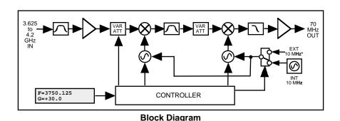
FIGURE 1.2 Model 2016-37 Downconverter Block Diagram
