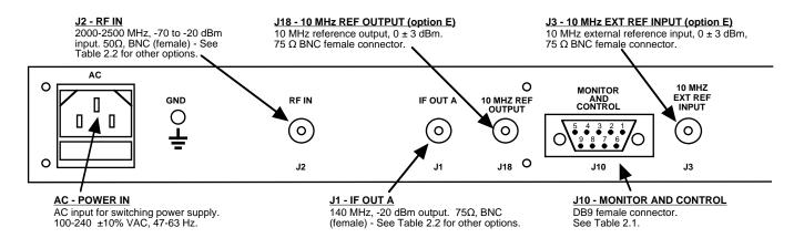
FIGURE 2.2 2016-26 Downconverter Rear Panel Inputs/Outputs
