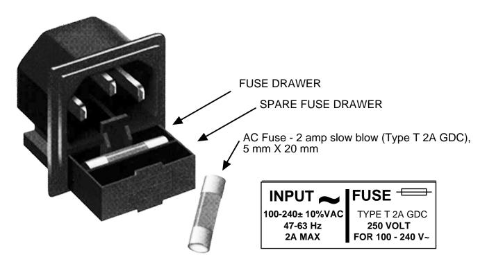
**FIGURE 2.4 Fuse and Spare Fuse Locations**
