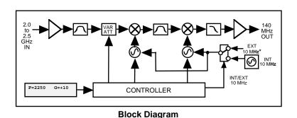
FIGURE 1.2 Model 2016-26 Downconverter Block Diagrams
