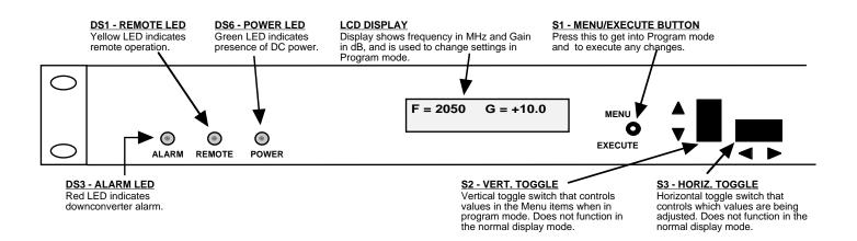
FIGURE 2.3 2016-26 Front Panel Controls and Indicators
