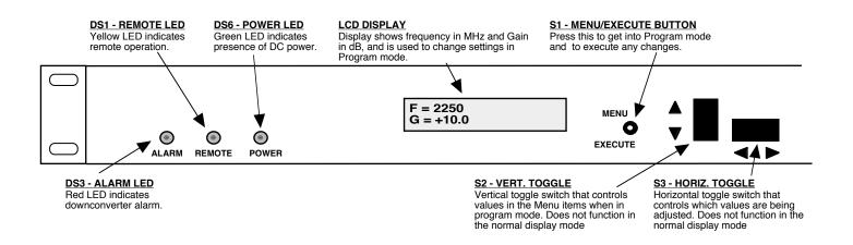
FIGURE 2.3 2016-25 Front Panel Controls and Indicators
