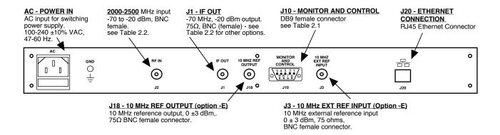
FIGURE 2.2 2016-25 Downconverter Rear Panel Inputs/Outputs
