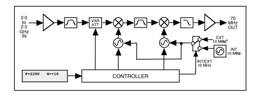
FIGURE 1.2 Model 2016-25 Downconverter Block Diagrams
