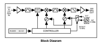
FIGURE 1.2 Model 2016-25-300 Downconverter Block Diagram
