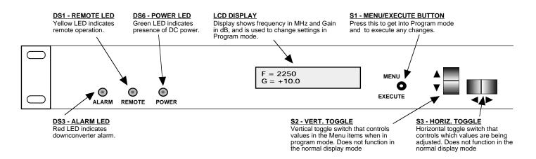
FIGURE 2.3 2016-25-300 Front Panel Controls and Indicators
