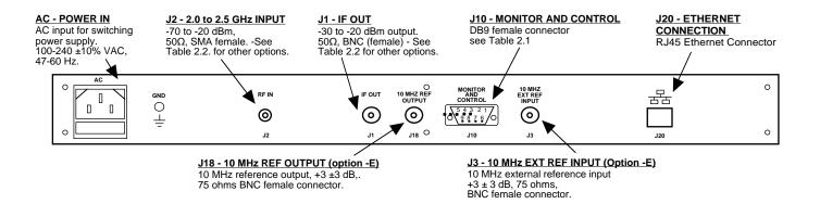
FIGURE 2.2 2016-25-300 Downconverter Rear Panel Inputs/Outputs
