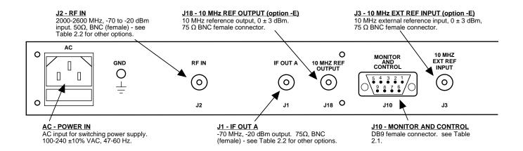
FIGURE 2.2 2016-2026 Downconverter Rear Panel Inputs/Outputs
