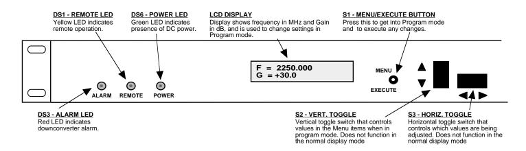
FIGURE 2.3 2016-2026 Front Panel Controls and Indicators
