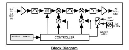
FIGURE 1.2 Model 2016-2026 Downconverter Block Diagrams
