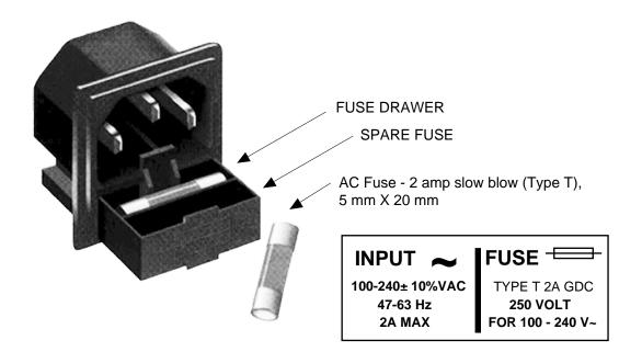
FIGURE 2.4 Fuse and Spare Fuse Locations
