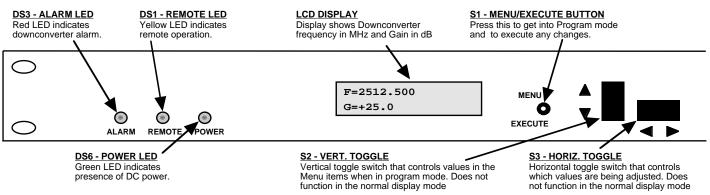
FIGURE 2.3 Front Panel Controls and Indicators
