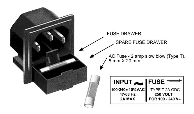
FIGURE 2.4 Fuse Location and Spare Fuse
