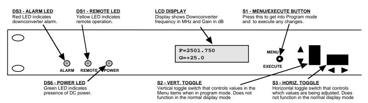
FIGURE 2.3 Front Panel Controls and Indicators
