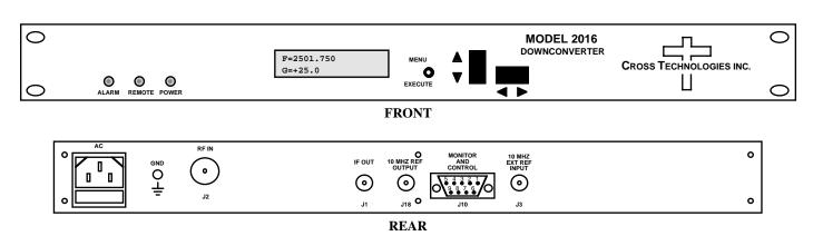
FIGURE 1.1 Front and Rear Panels
