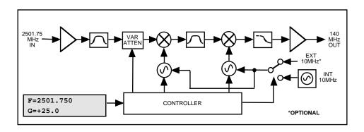
FIGURE 1.2 Block Diagram
