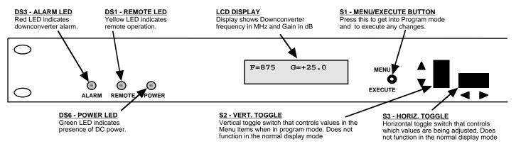
FIGURE 2.3 2016-10 Front Panel Controls and Indicators
