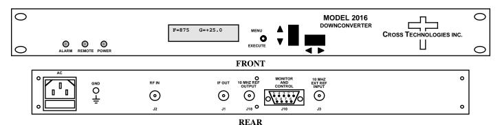
FIGURE 1.1 Front and Rear Panels
