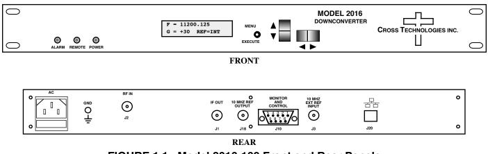
FIGURE 1.1 Model 2016-109 Front and Rear Panels
