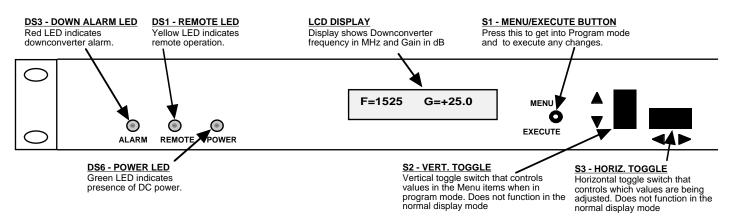
FIGURE 2.3 2016-05 Front Panel Controls and Indicators
