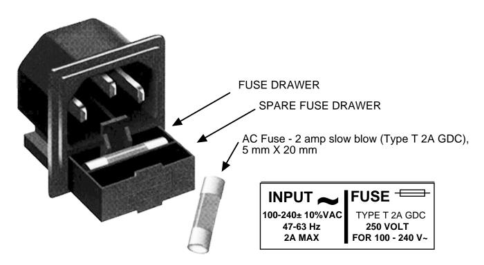
FIGURE 2.4 Fuse Location and Spare Fuse
