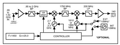
FIGURE 1.2 Model 2016-05 Downconverter Block Diagram
