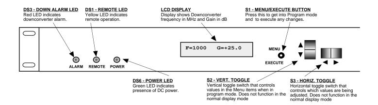
FIGURE 2.3 2016-0510 Front Panel Controls and Indicators
