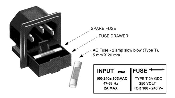
FIGURE 2.4 Fuse Location and Spare Fuse
