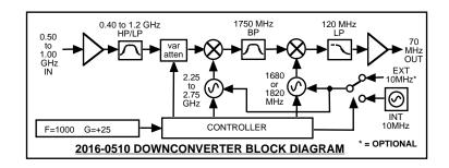
FIGURE 1.2 Model 2016-0510 Downconverter Block Diagram
