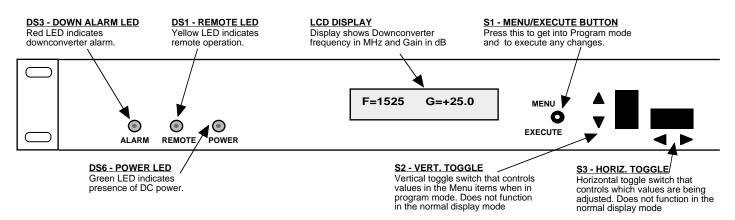
FIGURE 2.3 2016-04 Front Panel Controls and Indicators
