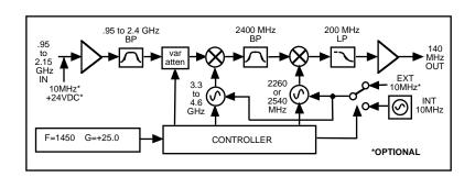
FIGURE 1.2 Model 2016-04 Downconverter Block Diagram
