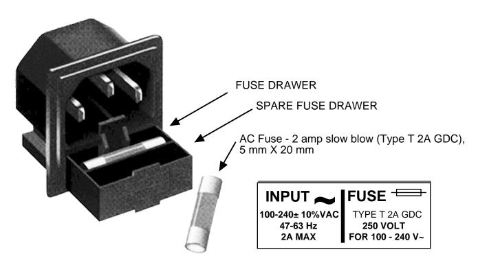
FIGURE 2.4 Fuse Location and Spare Fuse
