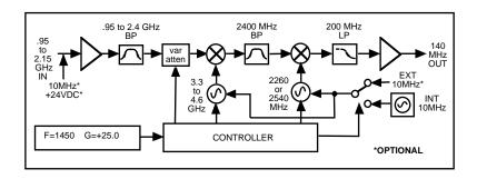
FIGURE 1.2 Model 2016-04A Downconverter Block Diagram
