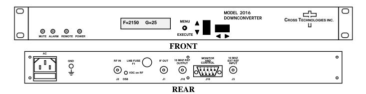
FIGURE 1.1 Model 2016-04A Front and Rear Panels
