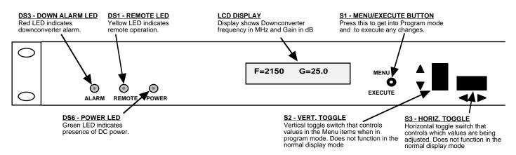
FIGURE 2.3 2016-04A Front Panel Controls and Indicators
