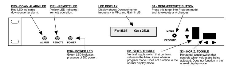
FIGURE 2.3 2016-03 Front Panel Controls and Indicators
