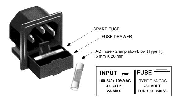
FIGURE 2.4 Fuse Location and Spare Fuse
