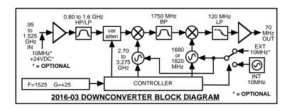
FIGURE 1.2 Model 2016-03 Downconverter Block Diagram
