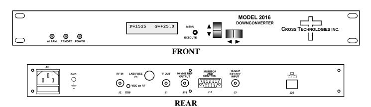
FIGURE 1.1 Model 2016-03 Front and Rear Panels
