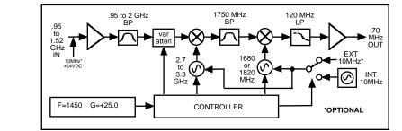
FIGURE 1.2 Model 2016-03A L-band Downconverter Block Diagram
