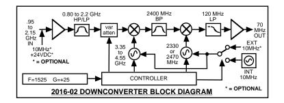
FIGURE 1.2 Model 2016-02 Downconverter Block Diagram
