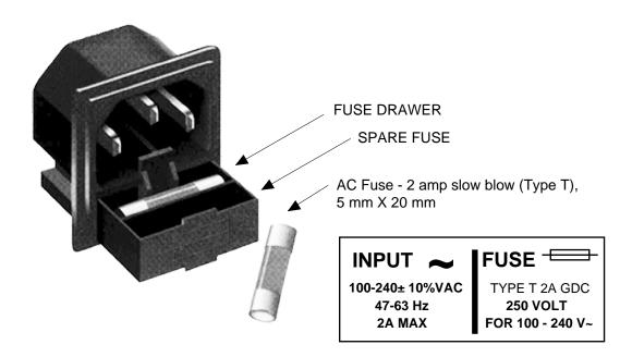
FIGURE 2.4 Fuse Location and Spare Fuse
