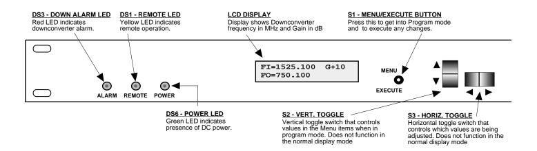
FIGURE 2.3 2016-02-790 Front Panel Controls and Indicators
