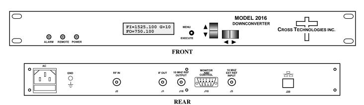
FIGURE 1.1 Model 2016-02-790 Front and Rear Panels (Optional Ethernet and LNB insertion shown)
