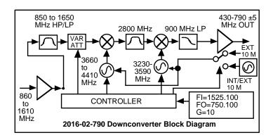
FIGURE 1.2 Model 2016-02-790 Downconverter Block Diagram
