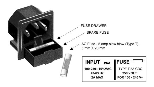
FIGURE 2.4 Fuse Location and Spare Fuse
