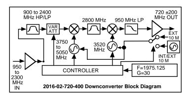
FIGURE 1.2 Model 2016-02-720-400 Downconverter Block Diagram
