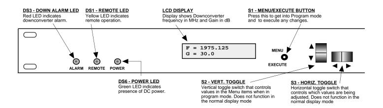
FIGURE 2.3 2016-02-720-400 Front Panel Controls and Indicators
