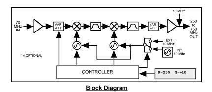
FIGURE 1.2 Model 2015-75 Upconverter Block Diagram
