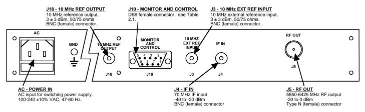
FIGURE 2.2 2015-61 Rear Panel Inputs and Outputs
