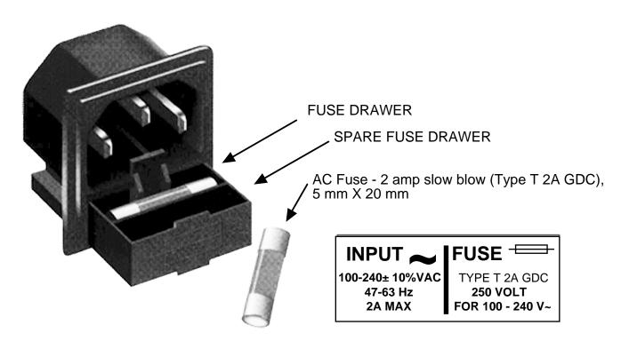
**FIGURE 2.4 Fuse Location and Spare Fuse**
