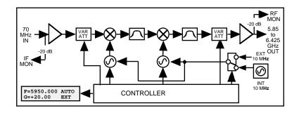
FIGURE 1.2 Model 2015-61 Upconverter Block Diagram
