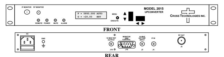
FIGURE 1.1 Model 2015-61 Front and Rear Panels
