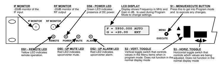
FIGURE 2.3 2015-61 Front Panel Controls and Indicators
