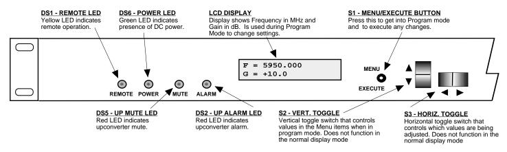
FIGURE 2.3 2015-58T Front Panel Controls and Indicators
