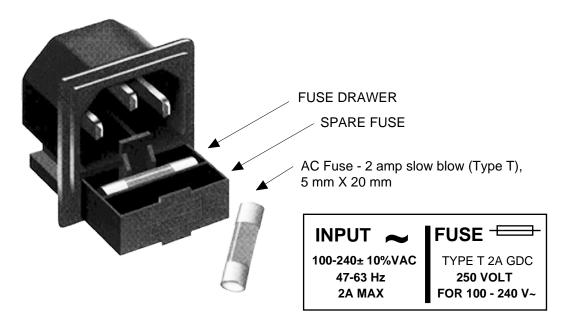
**FIGURE 2.4 Fuse Location and Spare Fuse**
