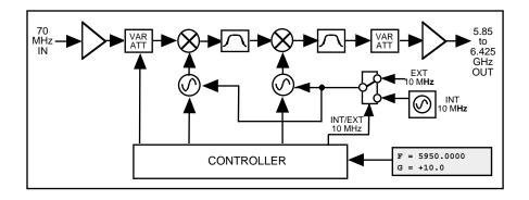
FIGURE 1.2 Model 2015-58T Upconverter Block Diagram
