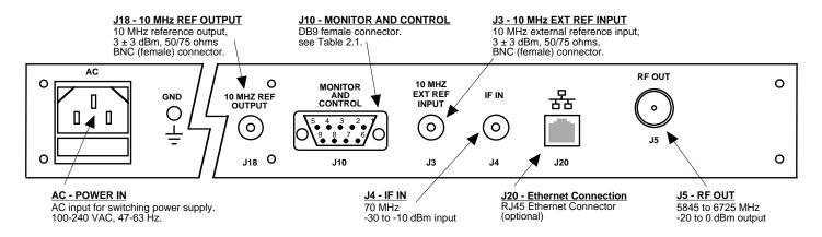
FIGURE 2.2 2015-58T Rear Panel Inputs and Outputs
