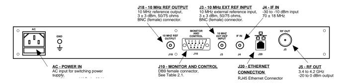
FIGURE 2.2 2015-35 Rear Panel Inputs and Outputs
