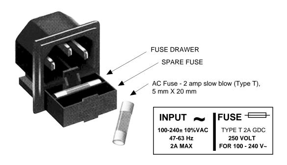
FIGURE 2.4 Fuse Location and Spare Fuse
