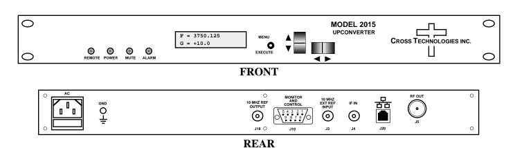
FIGURE 1.1 Model 2015-35 Front and Rear Panels (Shown above with Ethernet option)
