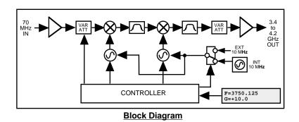
FIGURE 1.2 Model 2015-35 Upconverter Block Diagram
