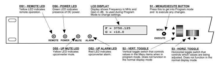
FIGURE 2.3 2015-35 Front Panel Controls and Indicators
