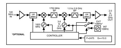
FIGURE 1.2 Model 2015-26 Upconverter Block Diagram
