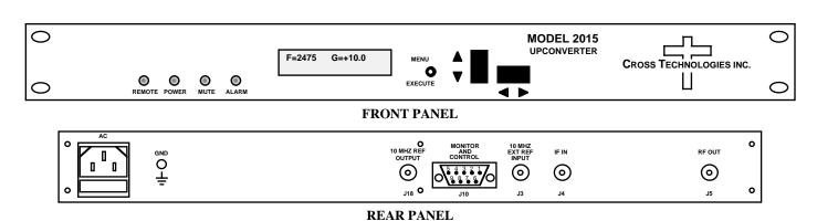
FIGURE 1.1 Model 2015-26 Front and Rear Panels
