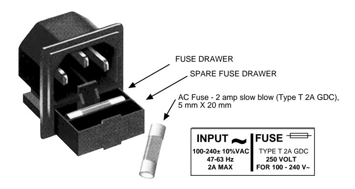
FIGURE 2.4 Fuse Location and Spare Fuse
