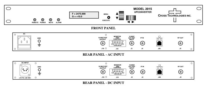
FIGURE 1.1 Model 2015-25 Front and Rear Panels
