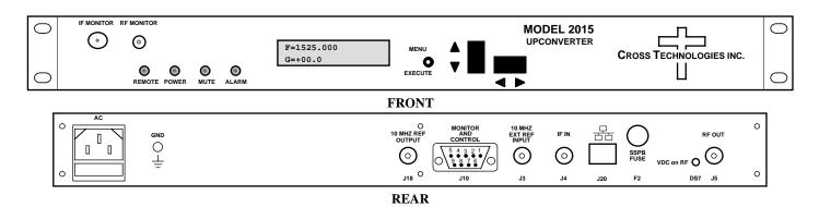
FIGURE 1.1 Model 2015-24 Front and Rear Panels
