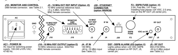
FIGURE 2.2 Rear Panel Inputs and Outputs
