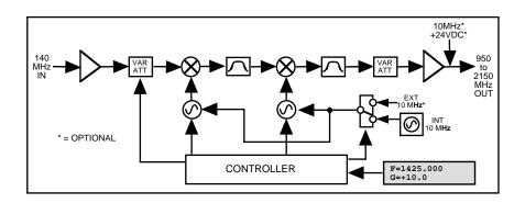
FIGURE 1.2 Model 2015-24 Upconverter Block Diagram
