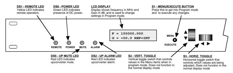
FIGURE 2.3 2015-152 Front Panel Controls and Indicators
