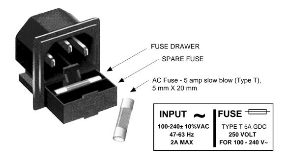
FIGURE 2.4 Fuse Location and Spare Fuse
