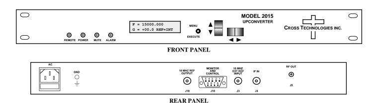
FIGURE 1.1 Model 2015-152 Front and Rear Panels
