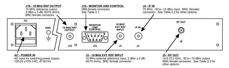
FIGURE 2.2 2015-152 Rear Panel Inputs and Outputs
