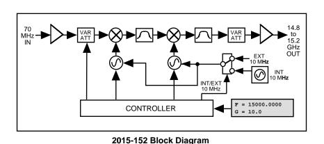
FIGURE 1.2 Model 2015-152 Upconverter Block Diagram
