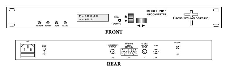
FIGURE 1.1 Model 2015-146 Front and Rear Panels
