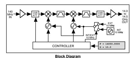
FIGURE 1.2 Model 2015-146 Upconverter Block Diagram
