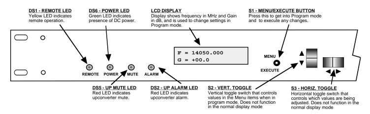
FIGURE 2.3 2015-146 Front Panel Controls and Indicators
