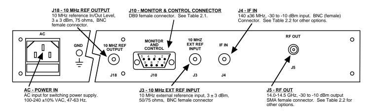
FIGURE 2.2 2015-146 Rear Panel Inputs and Outputs
