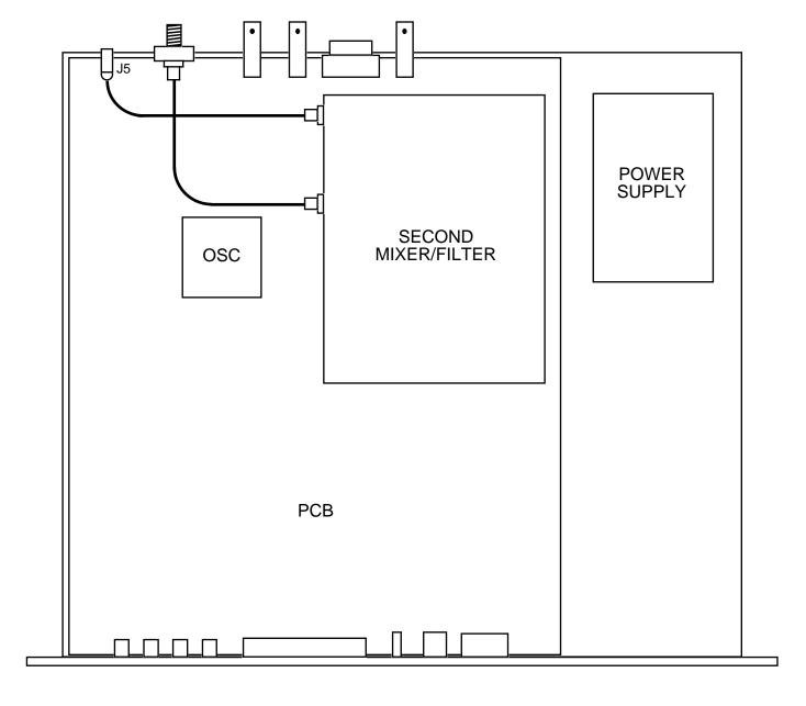
FIGURE 2.1 2015-146 Mechanical Assembly
