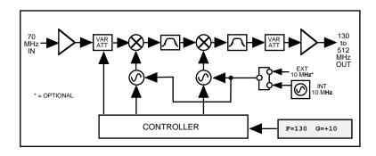
FIGURE 1.2 Model 2015-1351 Upconverter Block Diagram
