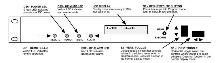
FIGURE 2.2 2015-1351 Front Panel Controls and Indicators
