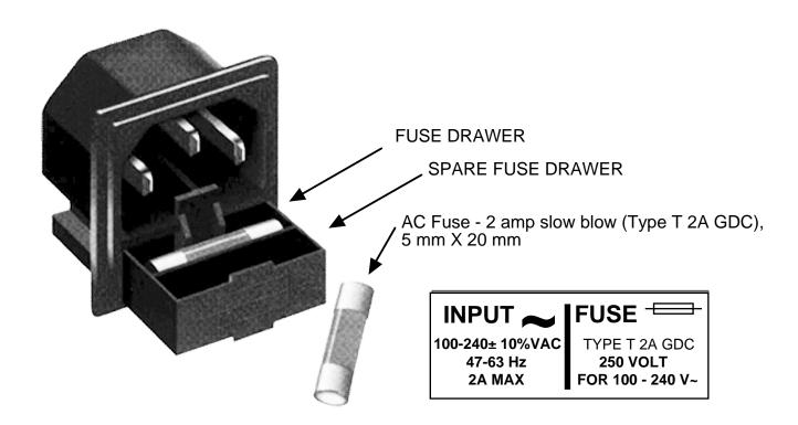
FIGURE 2.3 Fuse Location and Spare Fuse
