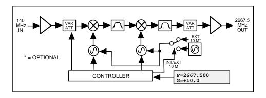
FIGURE 1.2 Block Diagram
