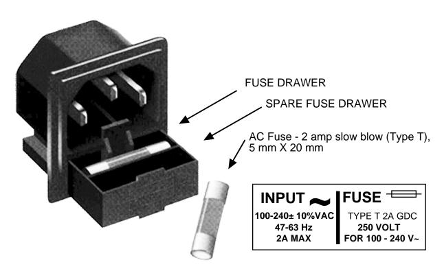
FIGURE 2.4 Fuse Location and Spare Fuse
