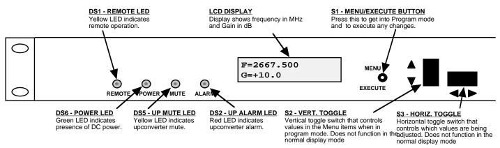
FIGURE 2.3 Front Panel Controls and Indicators
