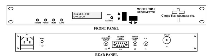
FIGURE 1.1 Front and Rear Panels
