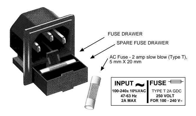
FIGURE 2.4 Fuse Location and Spare Fuse
