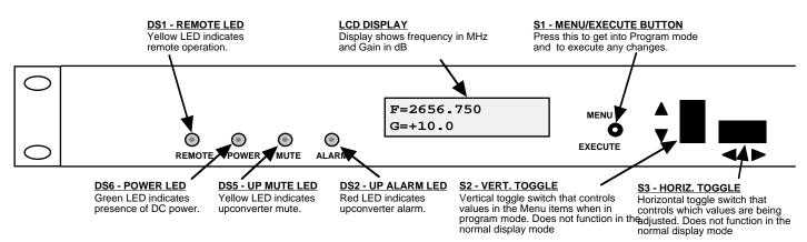
FIGURE 2.3 Front Panel Controls and Indicators
