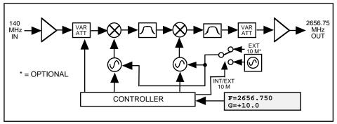
FIGURE 1.2 Block Diagram
