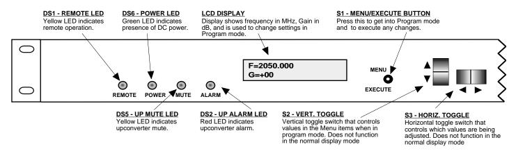
**FIGURE 2.3 Front Panel Controls and Indicators**
