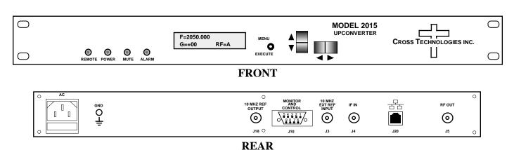
FIGURE 1.1 Model 2015-125 Front and Rear Panels
