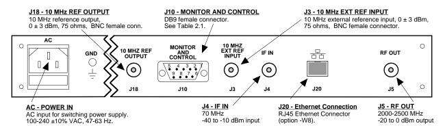
FIGURE 2.2 Rear Panel Inputs and Outputs
