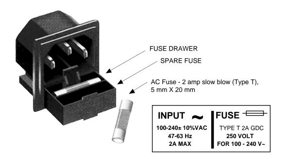
FIGURE 2.4 Fuse Location and Spare Fuse
