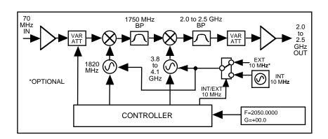
FIGURE 1.2 Model 2015-125 Upconverter Block Diagram
