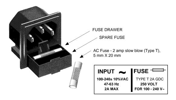
FIGURE 2.4 Fuse Location and Spare Fuse
