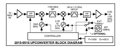
FIGURE 1.2 Block Diagram
