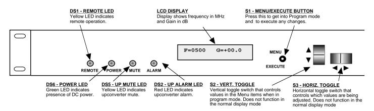
FIGURE 2.3 Front Panel Controls and Indicators
