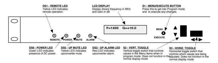
FIGURE 2.2 2015-03-01 Front Panel Controls and Indicators
