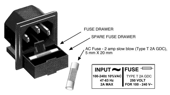
FIGURE 2.3 Fuse Location and Spare Fuse
