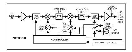
FIGURE 1.2 Model 2015-03-01 Upconverter Block Diagram
