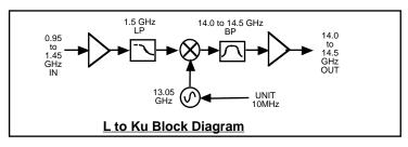
FIGURE 1.3 Model 2015-03U140 L to Ku Block Diagram
