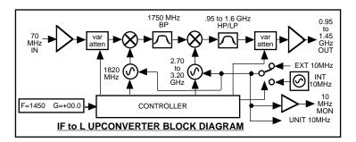
FIGURE 1.2 Model 2015-03U140 IF to L Block Diagram
