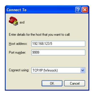
Figure 2.8: Telnet Settings in Hyper Terminal
