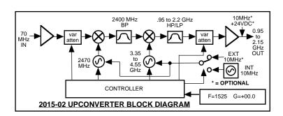
FIGURE 1.2 Model 2015-02 Upconverter Block Diagram
