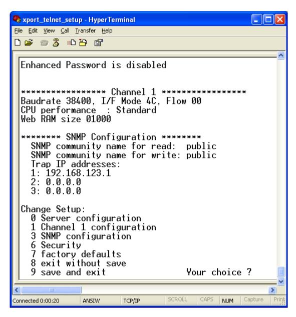
Figure 2.9: Device Server Configuration Menu
