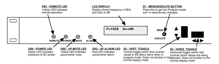
FIGURE 2.2 2015-02 Front Panel Controls and Indicators
