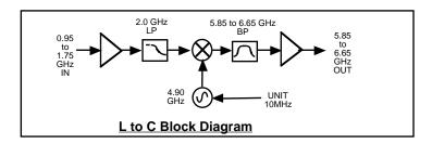
FIGURE 1.3 Model 2015-02U59 L to C Block Diagram
