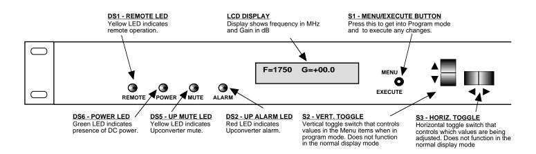
FIGURE 2.2 2015-02U59 Front Panel Controls and Indicators
