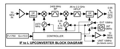
FIGURE 1.2 Model 2015-02U59 IF to L Block Diagram
